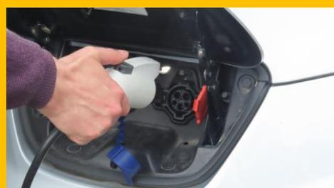
*Inserting the recharging plug.*
